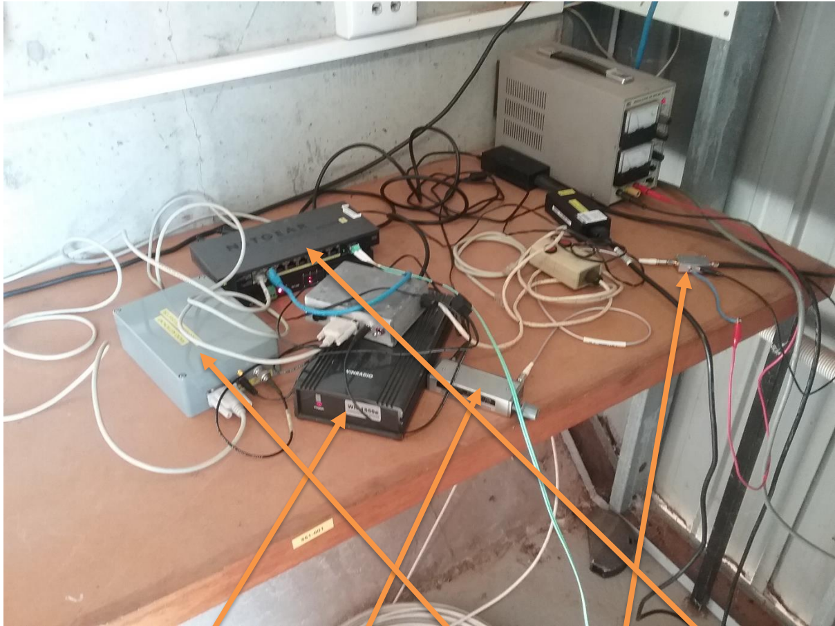
The receiver (a Win Radio 1550e), the attenuator, detector / integrator, bias T and network equipment.
