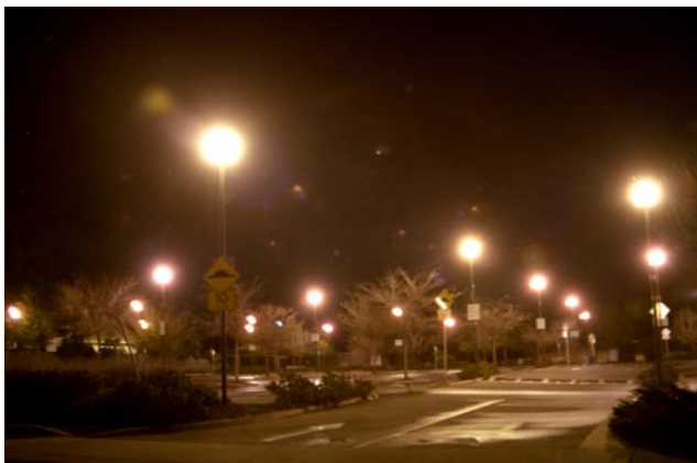
Glary globe-lights at a car park waste light sideways and upwards, and contribute to skyglow.
